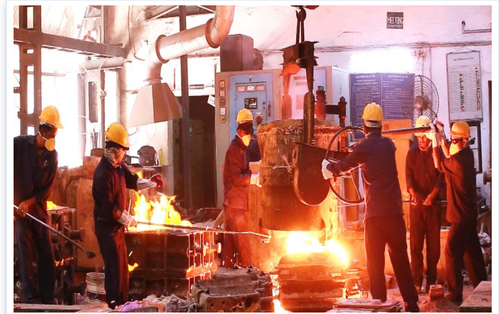
In-house induction melting with dual Spectro verification
